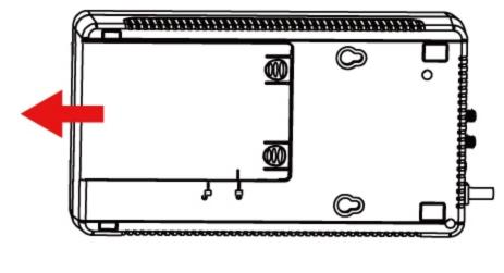
2. LIFT the battery out of the compartment, and disconnect wires from battery positive (+) and negative (-) terminals. Get a new battery and make sure to re-connect wires to positive and negative terminals correctly.
