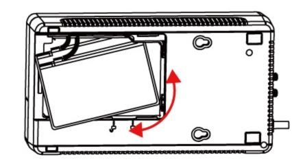
3. Slide the battery compartment cover back onto the battery housing. Double check if battery compartment is well-locked.
